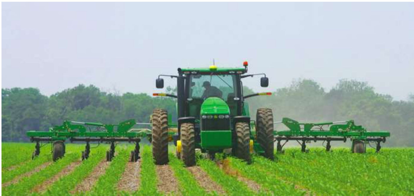
Side dressing with a John Deere 2510H Nutrient Applicator toolbar allows for minimal soil disturbance in this no-till field. It also splits nutrient applications to reduce leaching and improve nitrogen use by corn plants.
