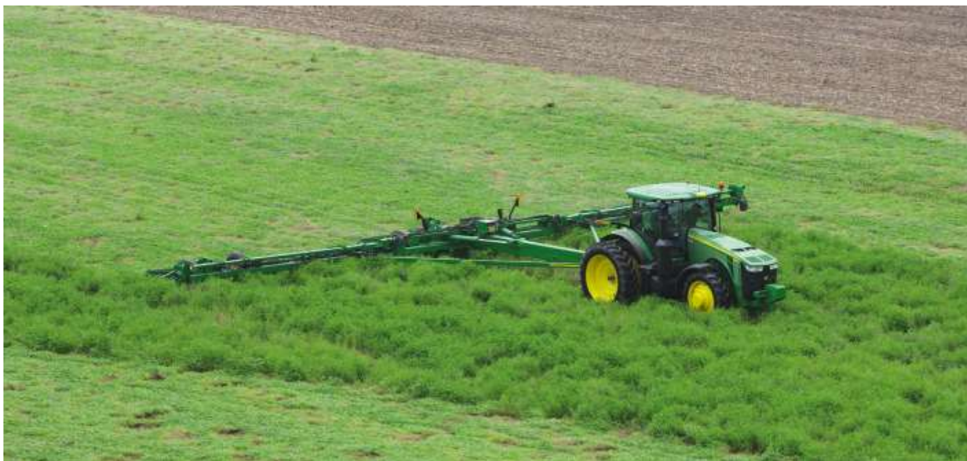
This custom-built 60-foot roller crimper helps to manage cover crops on commercial scale research farms. We believe this is the largest roller crimper in the world, designed on a John Deere 1770 NT tool bar to match up with a 24-row 1770 NT planter and to fold to 12-feet wide for transportation.
